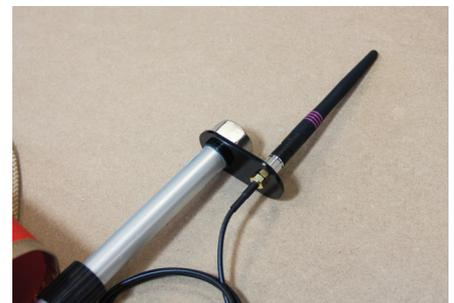
3. Refit telescopic pole to survey bar - routing SMA cable (A8) through to bag interior. Attach female connector on SMA cable (A8) to VBOX Telemetry module (G).
