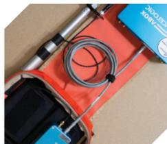
8. Connect the li-ion battery pack (A3) to the 'PWR' port on the VBOX 3i (F).
