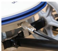
10. Connect the VBOX File Manager (E) to the VBOX 3i systems (F) 'CAN' port using a 5-pin LEMO cable (D).
