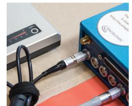
9. Link the GPS ground plane antenna (B) to the 'SATS' SMA connector on the VBOX 3i using the TNC to SMA cable (A1).
